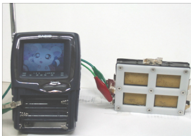
Fig. 9. Photograph of the eight-cell module powering a small TV-set.
